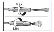
→ To apply detergent, the wand must be positioned to the lower pressure setting (Mix).
