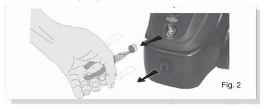
**Step 2**Connect the high pressure hose to the machine outlet. To connect, carefully insert the L-shaped connector fitting with the o-ring into the high pressure outlet and tighten the threaded nut by hand.
