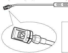
**Step 1** To apply detergents the triple jet nozzle must be set to the "CHEM" position.
