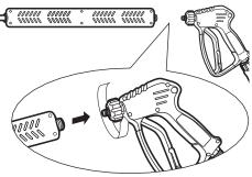
**Step 4** Attach the spray wand to the trigger gun.
