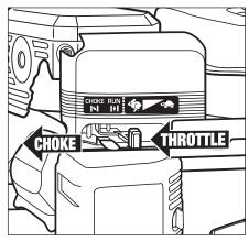
**Step 7** Slide the throttle control to the fast (Rabbit) position. Move the choke lever to the "CHOKE" position (only if the engine is cool). After starting, move the choke to "RUN".
