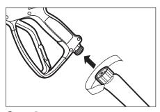
**Step 2** Attach high pressure hose to trigger gun.
