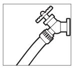
**Step 3** Connect garden hose to the cold water source and turn water on completely.
