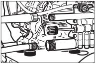
**Step 6** Disconnect the garden hose from the water inlet. Disconnect the high pressure hose from the high pressure outlet.
