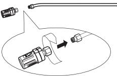
**Step 3** Attach the triple jet nozzle to the spray wand.
