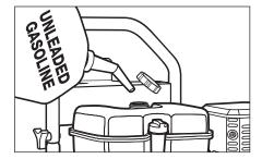
**Step 6** Fill gas tank with unleaded gasoline. Do not use leaded gasoline.
