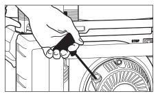
**Step 8** Pull the starter handle. If the engine fails to start after 3 pulls squeeze the trigger gun to release pressure, and repeat step 8.
